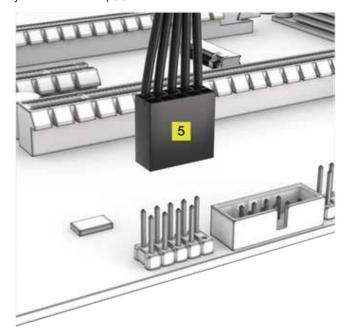
Connect the 9-pin USB 2.0 connector (5) into a USB 2.0 header on the motherboard.
