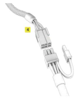
Connect the 6-pin PCIe connector (4) into a dedicated power cable from the power supply.
