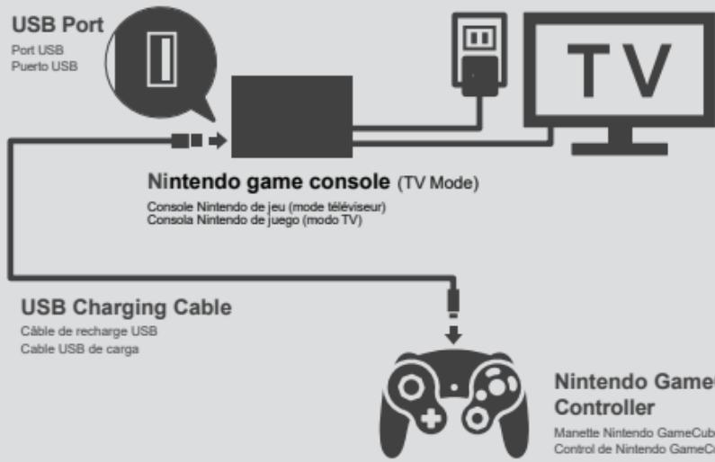
**The controller will automatically pair with the Nintendo game system when it is turned on in TV mode and connected with the USB Charging Cable.**
