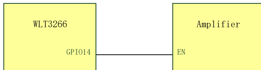
Figure 6. GPIO14 Reference design
