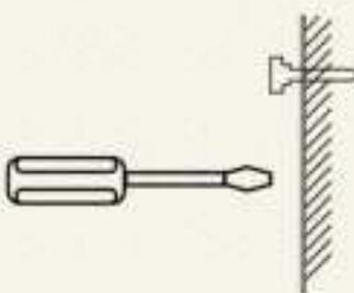
4 Insert the screws into the holes.
