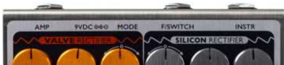
Rear connections. Right to left: Instrument input; External Footswitch; Power; Output
