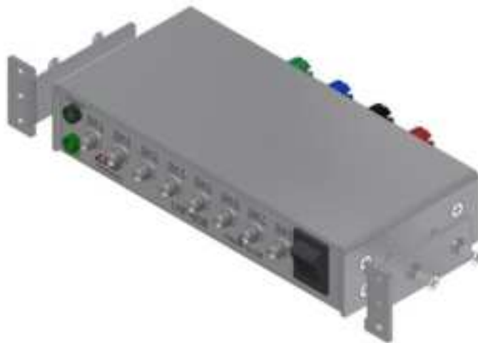
Figure 6 Attaching mounting flanges to LNF-BOB
