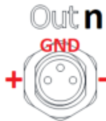
Figure 3 Out connector pinout - front view
