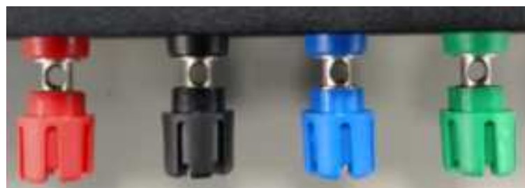
Figure 7 LNF-BOB Rear Plane - Binding Post Connectors
