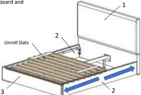
**STEP 6:** Verify the slats are installed properly the legs are perpendicular to the floor for full support.
