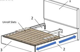
**STEP 6:** Verify the slats are installed properly the legs are perpendicular to the floor for full support.
