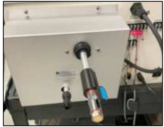
Figure 2-3 BC 1054 with Dilution System Inlet Location
