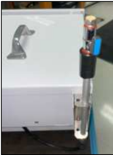
Figure 2-4 BC 1060 Inlet Location
