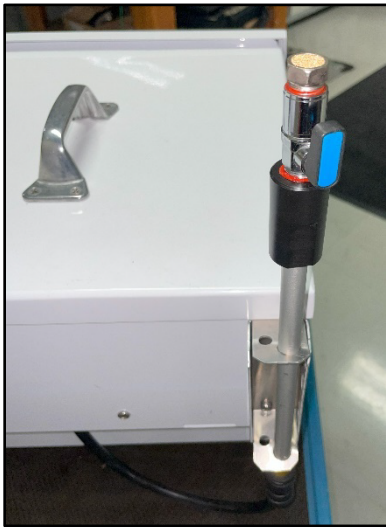
Figure 2-4 BC 1060 Inlet Location
