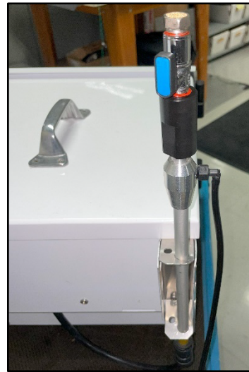
Figure 2-5 BC 1060 Inlet Location with Dilution Flow Adaptor
