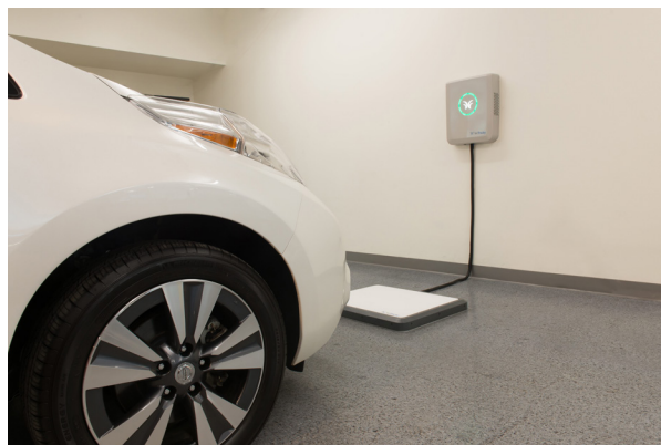
Figure 3: Home EV wireless charging system.
