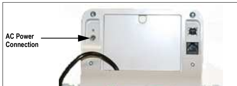
Figure 2-18. Power Connection Site
