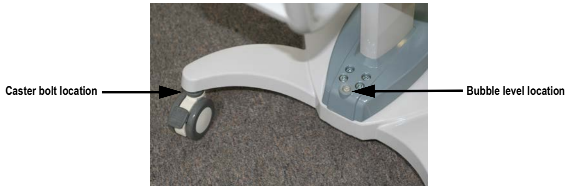
Figure 2-14. Bubble Indicates That The Scale is Level
