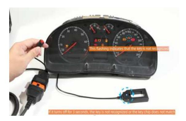
If the IMMO light on the instrument flashes, it means that the instrument has not recognized the key. If the induction adapter flashes for three seconds and then turns off, it also means that the key has not been recognized or the key chip does not match.
