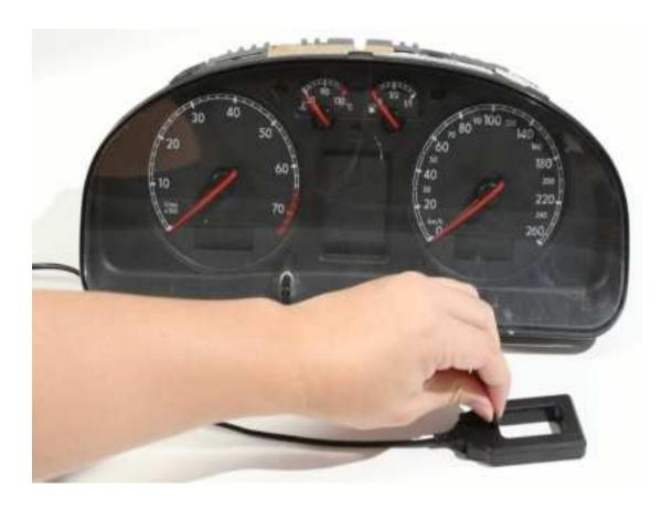
After pressing the ignition switch, you can see the light on the induction adapter flash quickly and then go out immediately, and the IMMO flash quickly and then go out immediately. This means that the chip is matched successfully.
