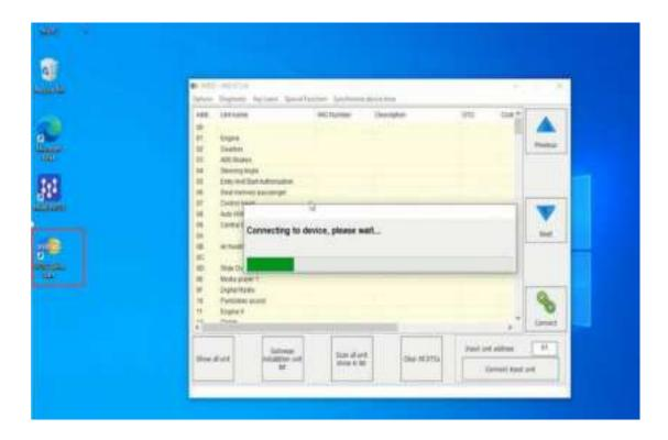
Step 3: Select"VW">>"K-Line Instrument/Immobox">>"Instrument Cluster(VDO66, VDO86, Motometer)">>"Read EEPROM">>"Save File".
