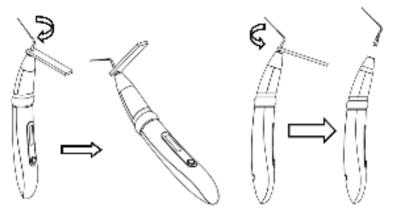
Tighten clockwise to install the tip
