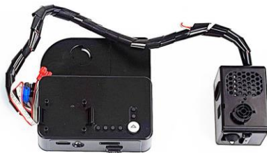
Control box and print head
