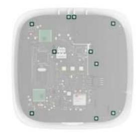
**6.** Carefully remove both boards, keeping them in the same plane and not disconnecting them. There is a connector between boards: do not break it.
