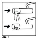
For the Pocket Tap Self-Priming (click valve tap). To activate the water flow, press the faucet from the front and hold.
