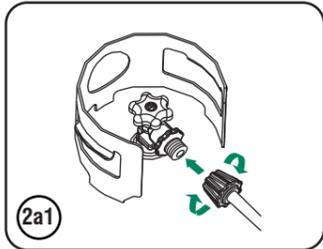
**Connect the LPG gas hose to the propane fuel source.**
