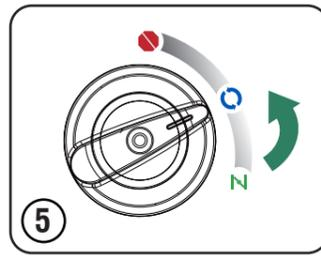
Turn the starting dial switch to the **RUN** **O** position.
