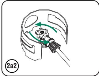
**Fully open the Propane/LPG cylinder knob.**
