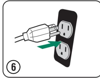
**Plug in items to be powered, using only grounded extension cords.**
