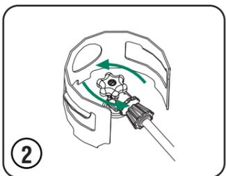
**Fully open the Propane/LPG cylinder knob.**
