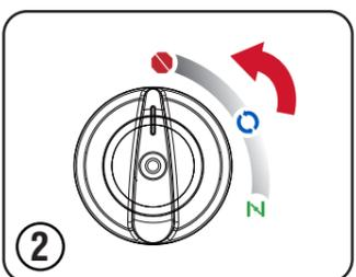
**Turn the starting dial switch to the OFF position.**
