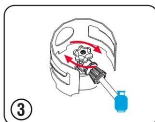
**Turn the fuel valve knob to the OFF position**
