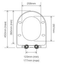
max/min fixing adjustment
