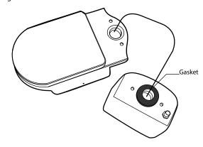
Insert the cistern fitting bolts arranging the components as shown in the diagram below.
