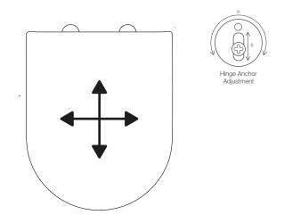
Adjust the position of the hinge anchors to make sure the seat lines up with the edges of the toilet pan.
