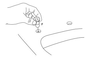
If difficult to push in, lubricate the rubber insert with water.
