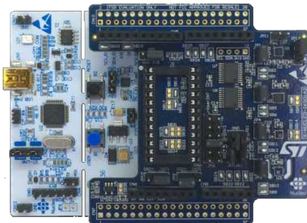
Figure 3. Sensor expansion board and adapter connected to the STM32 Nucleo
