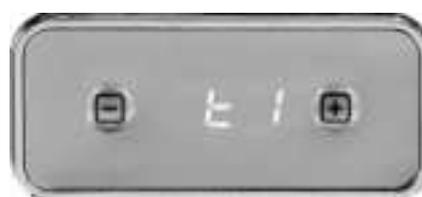
Now you can reduce the remaining time from the preset grinding time 't1' in tenths of a second by quickly pressing '-' (increase the time again with pressing '+').
