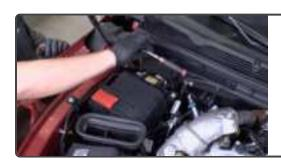
If you rush this step and unplug the MAP sensor, it can flag a Check Engine Light in the ECM on startup.
