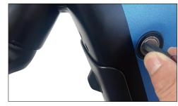
Ensure the bike is turned off. Insert the key and turn towards the ""unlock"" icon. The battery will pop out of its holding.
