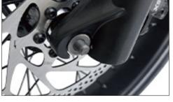
Insert the front wheel hub axle into the front wheel and secure them into the front fork.
