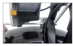
Install the mudguard and headlight in seauence.
