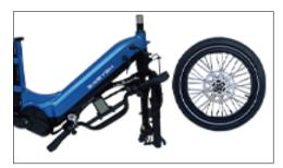
1 Remove the protective shield from the disc brake.
