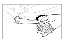
3 Thread the left pedal onto the left crank gently by hand, turning counter-clockwise. Then tighten the pedal with an Allen wrench.
