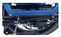
Remove the 8 screws on the left and right sides.
