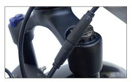
Plug in the headlight. Locate the two sides of the orange, three-pin headlight connector, carefully align the internal pins and notches and external arrows, then press directly together without twisting to fully seat the connection.
