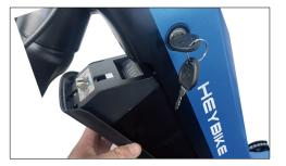
NOTE: The battery weighs roughly 10lbs and should be handled with care. Prop up the battery with your left hand and then remove the battery with both hands.
