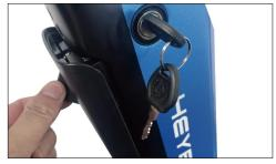
Hold the bike frame with one hand, and the locking device on the battery with the other. Turn counter-clockwise to unlock.
