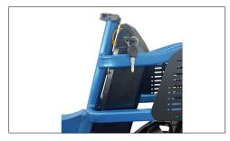
1 To remove the battery, turn the key to the UNLOCK position.
