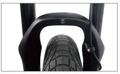
Remove the nut, washer and bolt at the top of the front fork.
