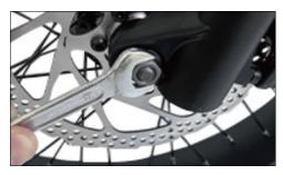
3 Assemble the screws and washers in the correct order and tighten both sides of the screws.
