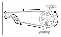
Check the chain alignment. Rotate the right pedal counter-clockwise. Watch the chain and ensure it runs through the drivetrain (the rear cog, chain tensioner, and around the front chain ring) smoothly.
