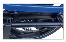
3 Pay attention to distinguishing the left and right footboards and aligning the installation holes.
