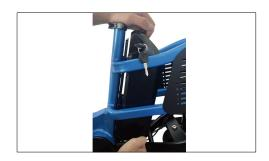
2 Then carefully pull the battery up until the battery detaches from the receptacle.
