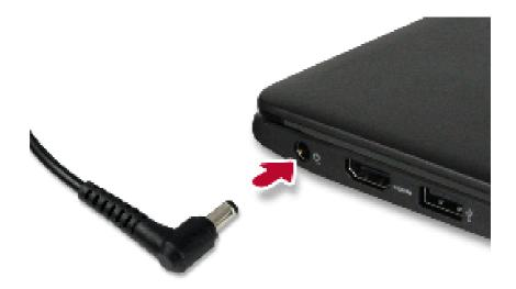
Open the LCD and check the charging state. When the AC adapter lamp is blinking, charge it fully with the AC adapter before using it.
