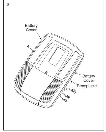
7. While a second person holds the Console (4) near the Upright (2), connect the wires on the Console to the Upright Wire (28) and to the Pulse Wires (63).
