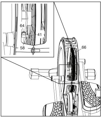
Next, rotate the Pulley (66) until a Magnet (41) is aligned with the Reed Switch (58). Slide the Reed Switch slightly toward or away from the Magnet. Then, retighten the M4 x 16mm Screw (64).
