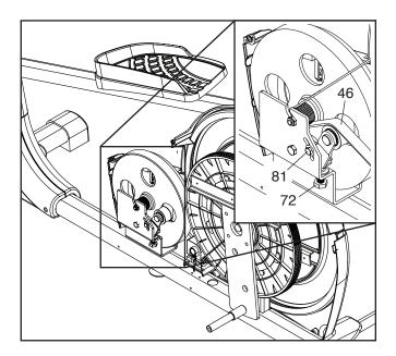
When the Drive Belt (46) is tight, tighten the Pivot Screw (81).
