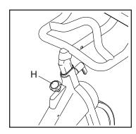
IMPORTANT: When the exercise bike is not in use, tighten the brake knob (H) completely.
