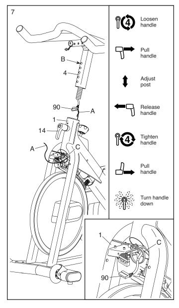
8. **See the inset drawing.** Connect the connector on the Handlebar Wire (90) to the connector on the Frame Wire (82).
