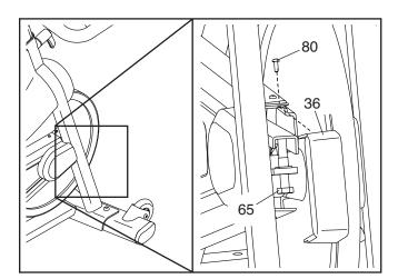
Then, tighten the M10 x 60mm Screw (65) until the Drive Belt (not shown) is tight.
