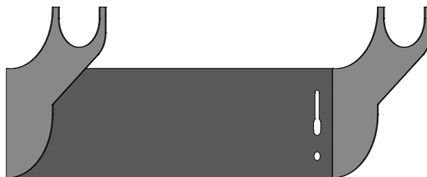
Figure 1-1: Upper mounting bracket for vertical Afinia radiators
