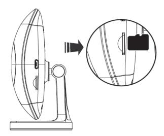
Make sure a Micro SD Memory card (Class 4 or higher, up to 32 GB) has been properly inserted into your Smart Security Cam. Micro SD Memory card not included and must be purchased separately. To properly insert the Micro SD Memory Card:
