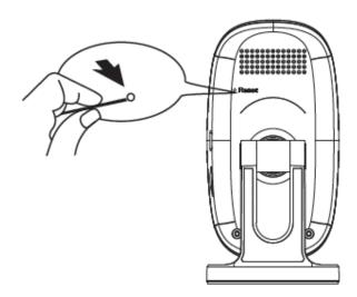
If the camera indicator is blinking blue upon startup, the camera needs to be reset. To reset the IP Camera:
