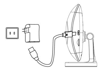
Connect one end of the Micro USB cable to your IP camera and the other end to the AC charger and then plug the AC charger into a power socket. The RED indicator light turns on.
