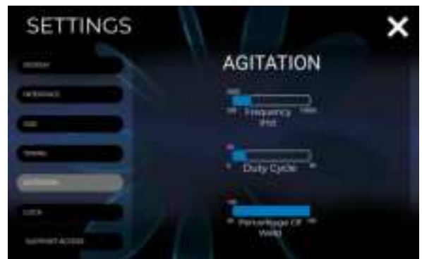
Figure 25.1. Use the Agitation Tab to make adjustments to the welder's energy agitation feature.
