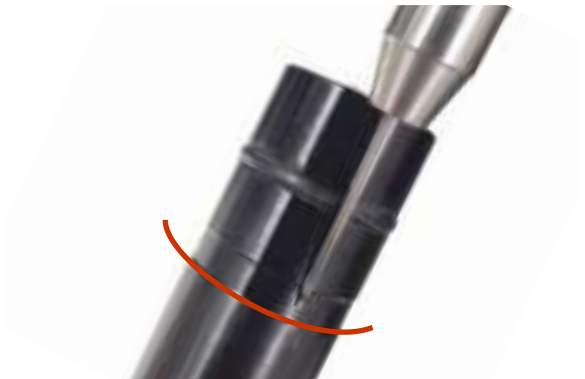
Figure 9.3. Use the guide engraved on the side of the stylus hull (E) for proper electrode (D) positioning.
