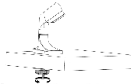
Figure 2.2. Lift Arm Assembly up and slide onto the table.
