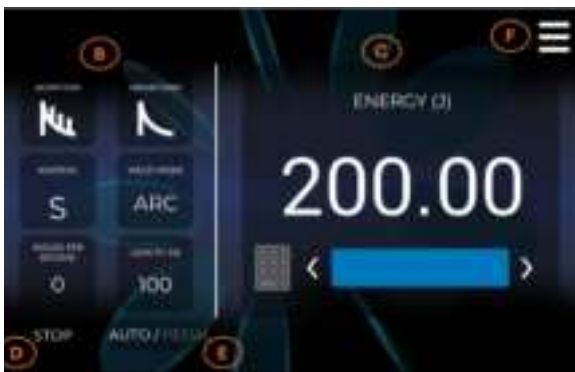
Figure 16.2. The Home Screen is divided into five sections: Widgets (B), Energy Adjustment (C), Stop Button (D), Trigger Selection (E), and the Menu (F)
