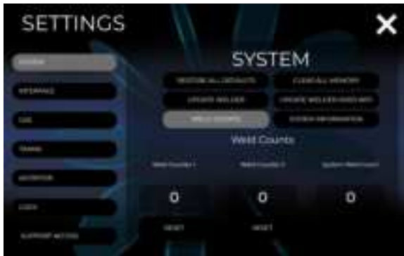
Figure 22.1. The welder will track three different weld counts: Weld Counter 1, Weld Counter 2, and System Weld Count.
