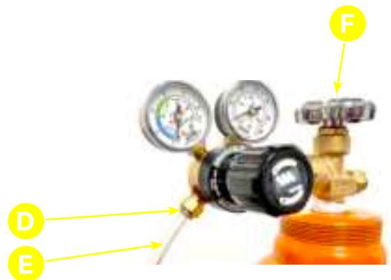
Figure 13.2. Connect the OD gas tube (E) from the power supply to the gas regulator port (D).
