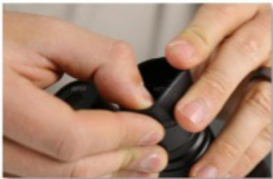
Figure 4.3. Push the two rubber eyepiece covers over the top of the microscope lenses.
