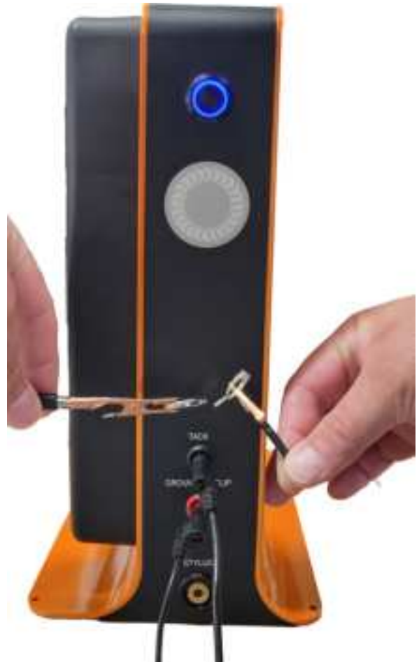
Figure 37.1. In Tack Mode, connect one ground to the Tack Port and another ground to the Grounding Clip Port on the front of the welder.
