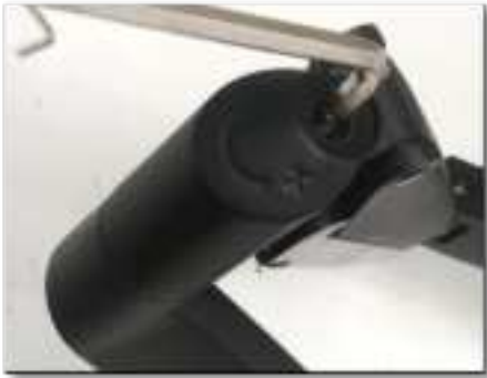
Figure 4.2. Adjust the tension of the Arm Assembly for more loose or more tight movement.
