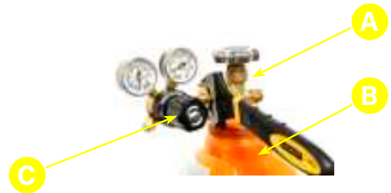
Figure 13.1. First, turn the regulator dial (C) counterclockwise to close the regulator valve. Screw the gas regulator (A) to the top of the shielding gas tank (B).
