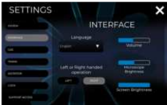
Figure 22.2. Use the Interface Screen to make adjustments to volume, microscope brightness, language selection, and left- or right-hand formatting.
