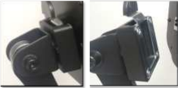
Figure 4.1 Though the screen case comes pre-attached, it can be removed by pulling the tab away from the screen.
