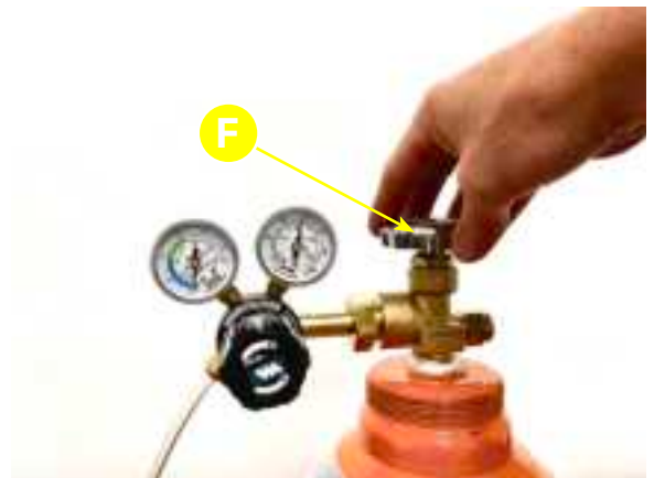
Figure 13.3. Open the shielding gas tank main valve (F) slowly clockwise until the left dial on the regulator port indicates gas pressure of 7-10 liters per minute.
