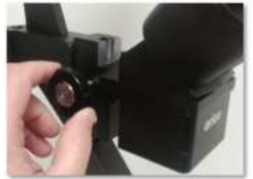
Figure 5.1. To adjust focus, turn the knob to move the optics up or down.
