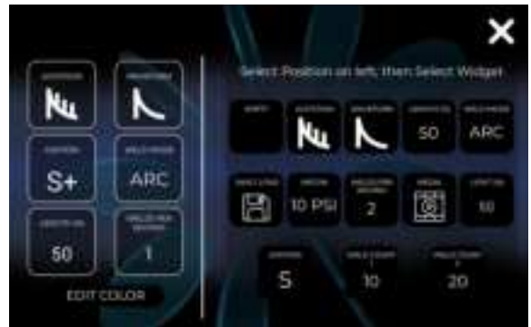
Figure 27.1. The Customize Screen allows you to change which widget you wish to appear on the Home Screen. You can also change the background color here.
