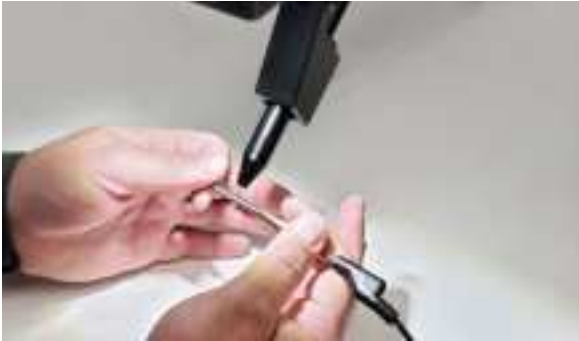
Figure 14.1. Rest your hands on the table and position the workpiece close to, but not touching the electrode., Then look through the microscope.
