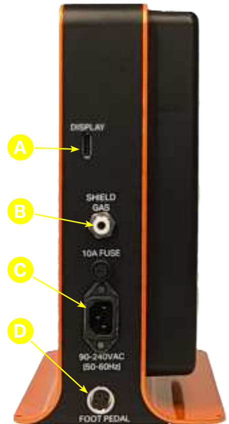
Figure 7.1. Connect the Comm Cable to the Display Port (A). Insert 1/4" gas tube into the Shield Gas Port (B). Plug the female end of the power cable into the 90-250VAC Port (C). Plug the foot pedal cable into the Foot Pedal Port (D).
