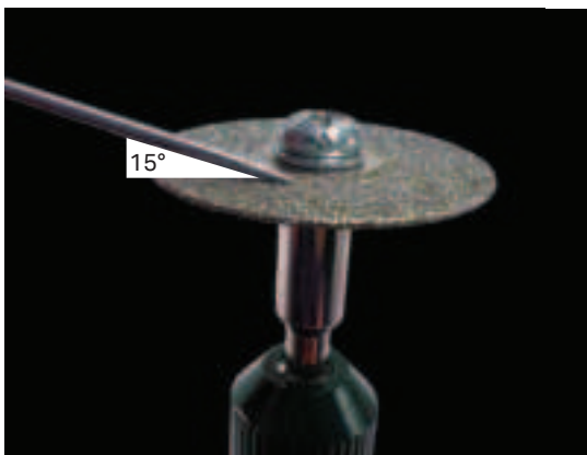
Figure 10.2. Use a rotary tool to sharpen the electrode.
