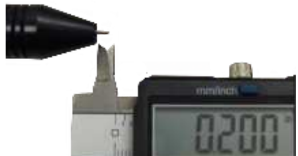
Figure 9.4. The electrode should protrude past the stylus hull (E) 1/8 to 1/4 inch (3.175 to 6.35 mm).
