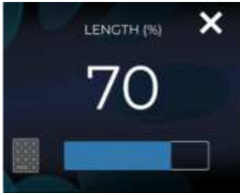
Figure 31.1. The Length Slider allows you to adjust the amount of discharge time for the weld.
