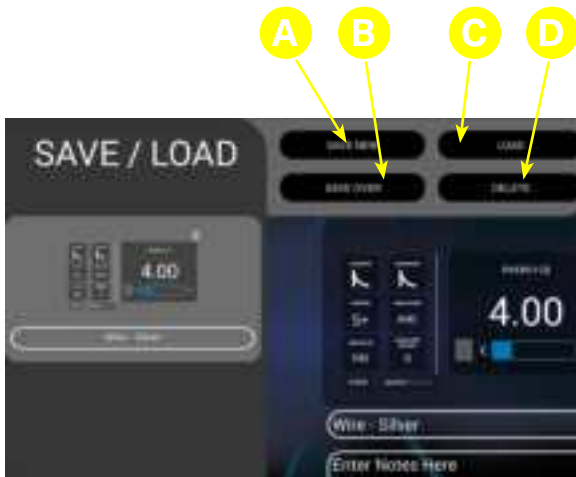
Figure 20.1. Use the Save/Load Screen to save favorite weld settings for future use. Saved welds can accessed or deleted here.
