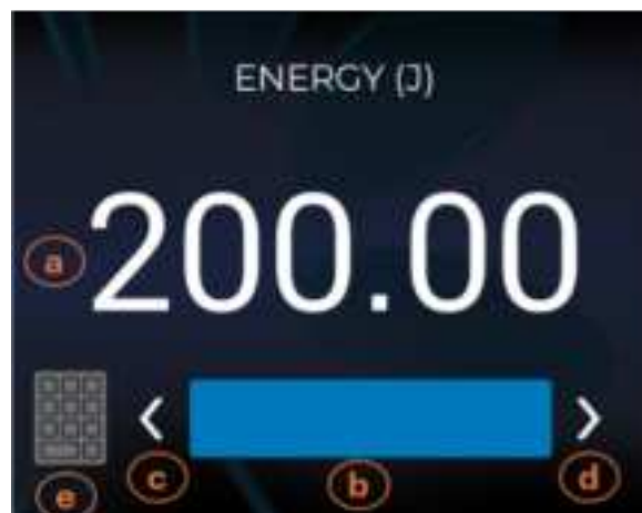
Figure 17.1. The current weld energy (a), i.e., the amount of energy to be released by the welder to the electrode, is displayed in the Energy Adjustment section. You can adjust energy in four different ways: Energy Slider (b); Left Button (c) and Right Button (d), Keypad (e), or the PowerNudge buttons shown in Figure 15.1.
