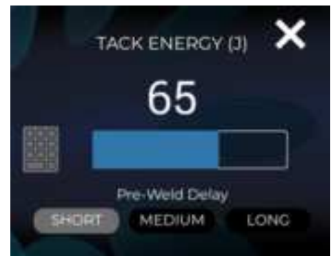
Figure 37.2. The Tack Controls appear when you press the Weld Mode Widget button and select Tack.
