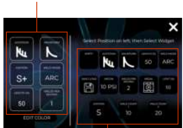
Figure 27.2. To customize the Home Screen, first select widget position you wish to assign on the left side of the Customize Screen.
