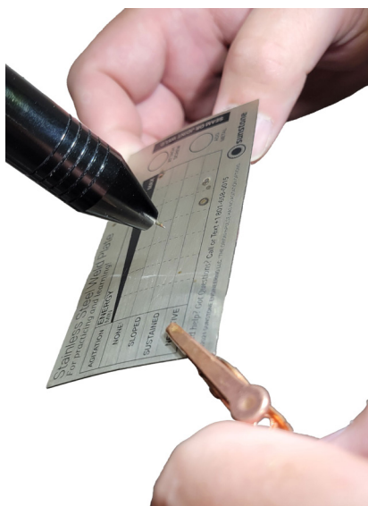
Figure 36.3. Attach the grounding alligator clip to the stainless steel welding plate.
