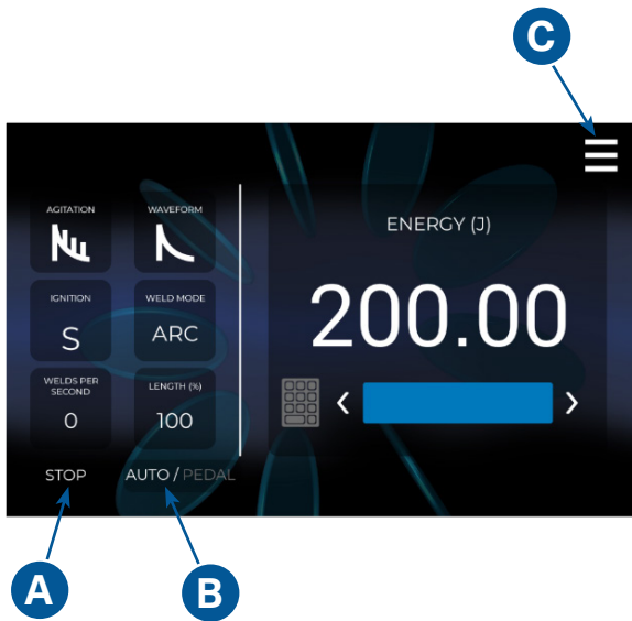
Figure 18.1. Location of the Menu, Stop, and Triggers Buttons.
