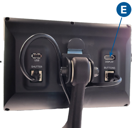
Figure 7.2. Connect the loose end of the Comm Cable into the Display Port (E) found on the back of the Screen Case.
