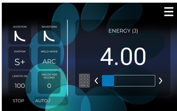
Figure 36.2. The Home Screen is where you will set welding parameters, such as energy, agitation, length, etc.
