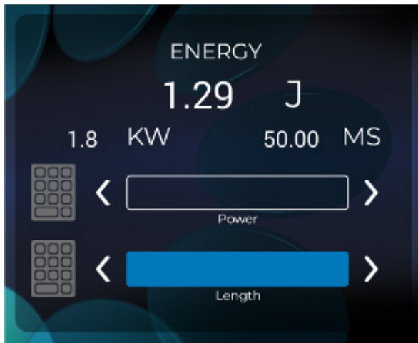
Figure 29.1. The Waveform Adjustment widget, only available with the Orion 200x, lets you control how energy is discharged, particularly helpful when working with difficult metals.
