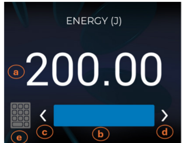
Figure 17.1. The current weld energy (a), i.e., the amount of energy to be released by the welder to the electrode, is displayed in the Energy Adjustment section. You can adjust energy in four different ways: Energy Slider (b); Left Button (c) and Right Button (d), Keypad (e), or the PowerNudge buttons shown in Figure 15.1.
