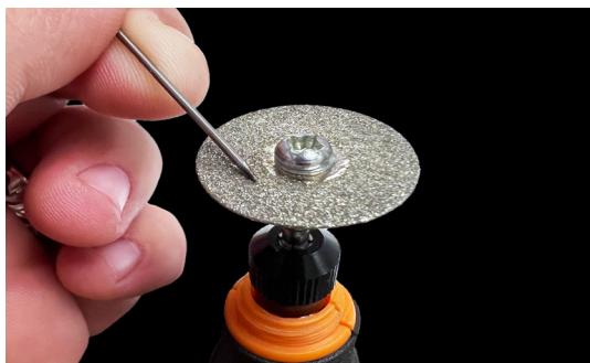
Figure 10.1. A sharp electrode tip improves arc initiation and results in a better overall weld.
