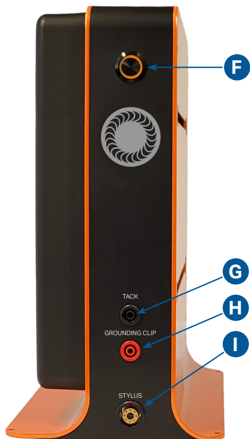
Figure 8.1. Connect the Stylus cord to the Stylus Port (I). Insert the alligator clip ground to the Grounding Clip Port (H). For the Orion 200x model, connect an additional ground to the Tack Port (G). Turn the welder on by pushing the Power Button (F).
