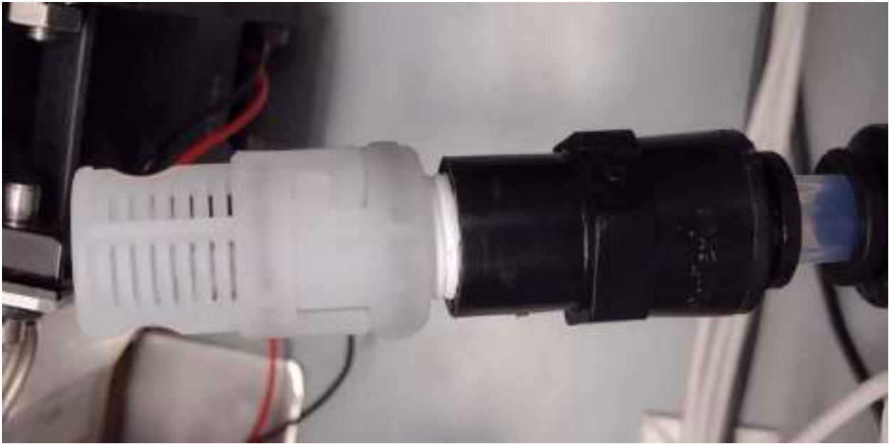
Figure 4: Vacuum Prevention Device
