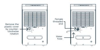
**Note:** Do not use this operation when the outdoor temperature is equal to or less than 32°F (0°C), otherwise the water will freeze, causing the water hose to block up and the dehumidifier may be damaged.
