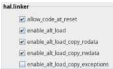
Figure 107. hal.linker Settings for QSPI Flash
