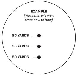
The top dot will be the shortest yardage; it is recommended to sight this in at 20 yards as described in the previous section. To set the second dot, gradually move your target out further until your POI and PDA are both in the center of the bullseye using the second dot (noting the yardage when this occurs). Repeat this process for the third dot.
