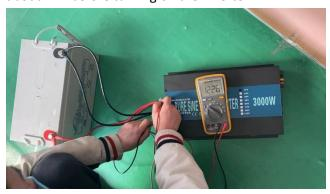
d.After turning on the inverter, confirm whether the LED display normally displays the input and output voltages.
