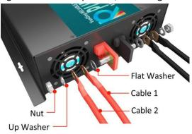
c.Use a multimeter to confirm the inverter input voltage. Make sure the voltage reaches about 12V before turning on the inverter.
