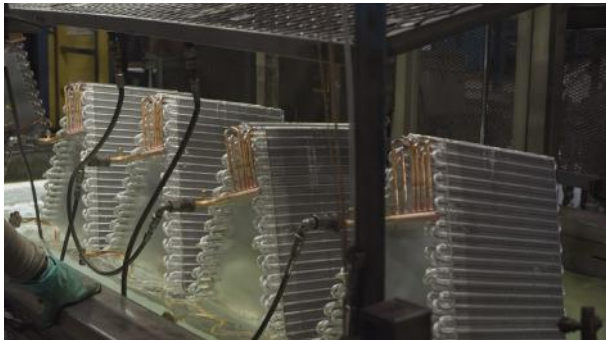
AIR UNDER WATER TESTING
