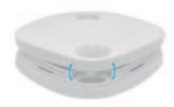
4 Pull up and open the battery cover in the back of the ATUVOS TAG.
