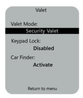
When the desired Valet Mode is displayed, press **FUNCTION** to save and transmit the command. When the command is received at the vehicle, a confirmation tone will play, and the cursor will exit the feature. The Valet text will now be displayed to identify the current system status. If the command fails to execute at the vehicle, the text will revert to OFF and error tone will play.
