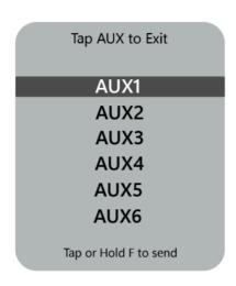
**LOCK** and **UNLOCK** are used to navigate up and down through available AUX outputs. When the intended AUX is highlighted, press **FUNCTION** to activate the output. For extended AUX commands (validity) continue holding the **FUNCTION** button for the desired duration.
