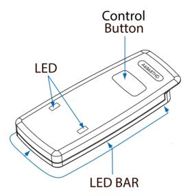
The Control Center, typically located on the upper part of the front windshield. It consists of:
