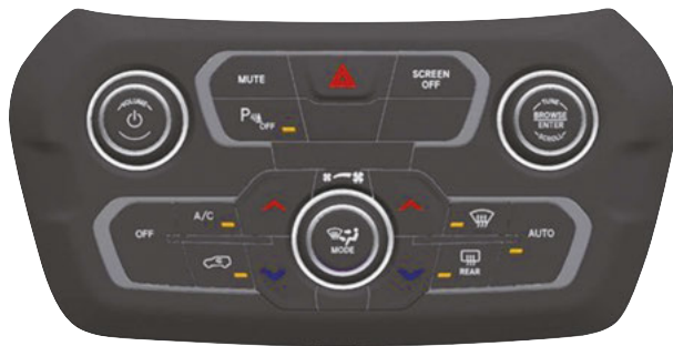
Automatic Temperature Controls (ATC)
