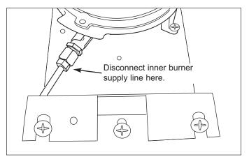
Figure 4-3. Disconnect Inner Burner Supply Line
