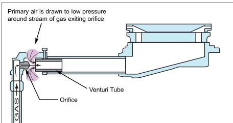
Figure 2-5. Gas Orifice
