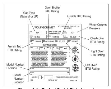
Figure 1-1. Typical Serial Plate Layout
