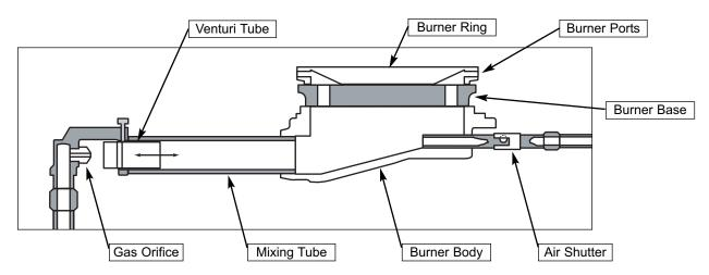
Figure 2-1. Cut-away View of Open Surface Burner Components
