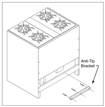
Figure 3-2. Anti-Tip Wall Bracket Installation
