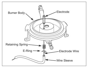
Figure 4-6. Surface Burner Electrode Removal
