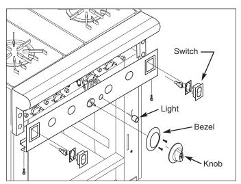
Figure 4-21. Switch, Light and Thermostat Removal
