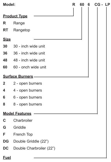
**LP** Propane Gas (*Propane Gas will be indicated by -LP* at the end of the model number. Example: R606CG-LP-LP)
