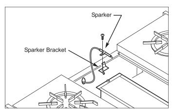
Figure 4-16. IR Griddle Sparker Removal
