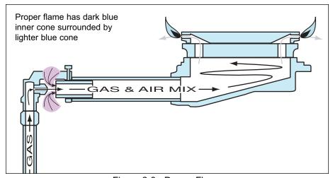
Figure 2-8. Proper Flame
