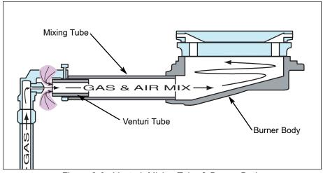
Figure 2-6. Venturi, Mixing Tube & Burner Body
