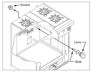
Figure 4-30. Light Components Removal
