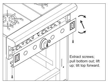
Figure 4-20. Control Panel Removal
