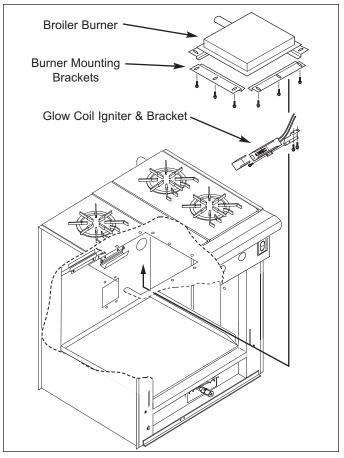
Figure 4-35. Broiler Burner & Igniter Removal
