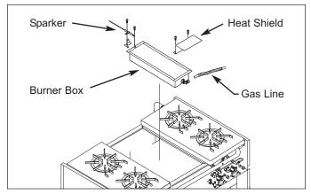
Figure 4-10. IR Charbroiler Burner & Sparker
