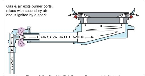
Figure 2-7. Gas/Air Exit Burner Ports and is Ignited
