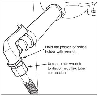
Figure 4-4. Disconnect Outer Burner Supply Line
