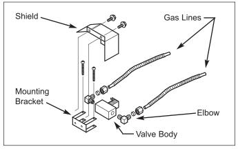
Figure 4-14. IR Griddle Solenoid Removal
