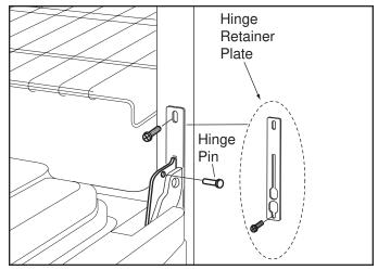
Figure 4-39. Hinge pin and retainer plate (SWS 17000000)
