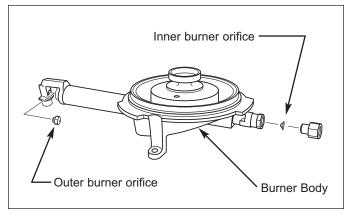
Figure 4-5. Surface Burner Orifice Removal
