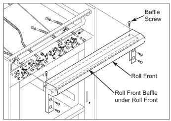
Figure 4-23. Roll Front Removal
