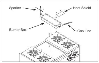
Figure 4-13. IR Griddle Burner Box Removal
