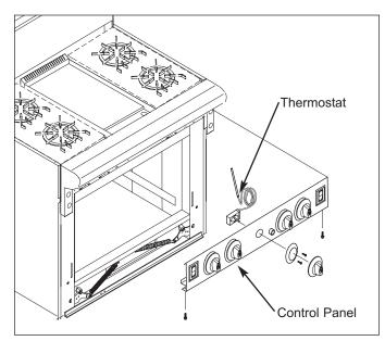
Figure 4-15. IR Griddle Thermostat Removal
