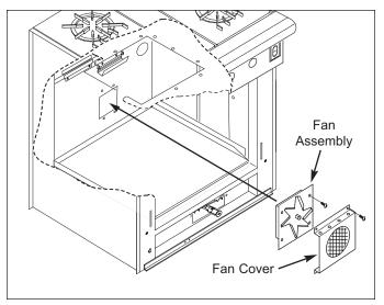
Figure 4-31. Convection Fan Removal
