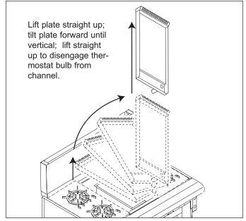
Figure 4-11. Griddle Plate Removal
