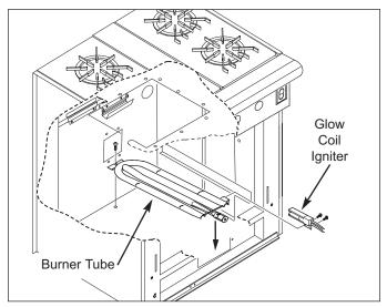
Figure 4-34. Burner Tube & Igniter Removal
