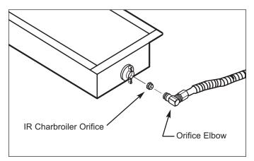
Figure 4-9. IR Charbroiler Orifice Removal
