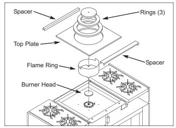
Figure 4-17. Components that Lift Off
