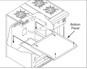
Figure 4-32. Bottom Panel Removal
