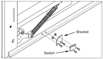
Figure 4-27. Door Switch Removal (PTS 17000000)
