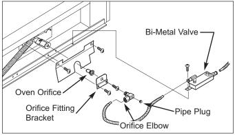
Figure 4-29. Oven Bi-Metal Valve and Oven Orifice Removal
