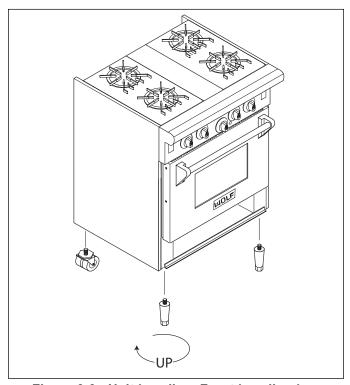
Figure 3-3. Unit Leveling, Front Leveling Leg
