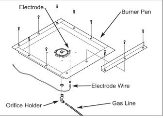
Figure 4-18. French Top Burner Pan Removal
