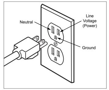
Figure 3-1. Proper Polarity at Electric Receptacle
