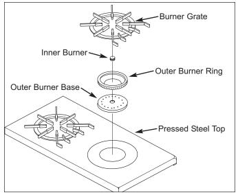
Figure 4-1. Components that Lift Off
