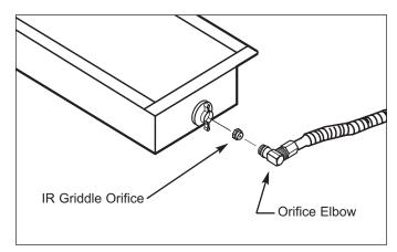
Figure 4-12. IR Griddle Orifice Removal
