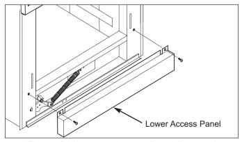
Figure 4-26. Lower Access Panel Removal
