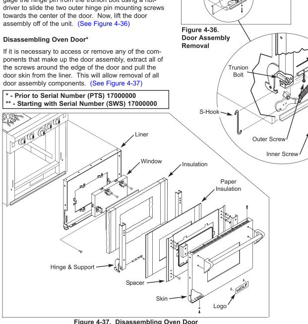
Figure 4-37. Disassembling Oven Door
