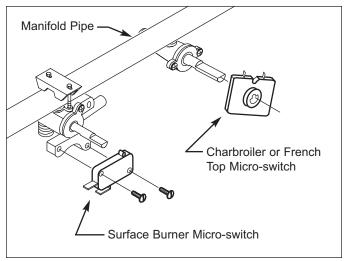
Figure 4-22. Micro-Switch Removal
