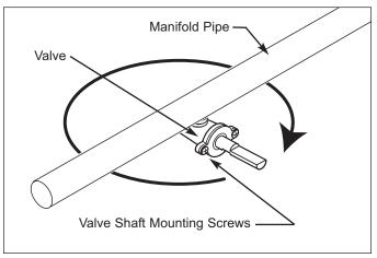
Figure 4-25. Charbroiler / French Top Valve Removal
