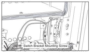
Figure 4-28. Door Switch Removal (SWS 17000000)
