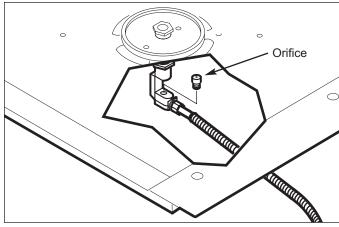
Figure 4-19. French Top Orifice Removal
