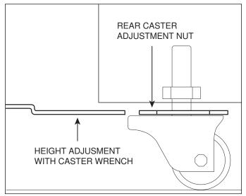
Figure 3-4. Unit Leveling, Rear Caster Adjustment
