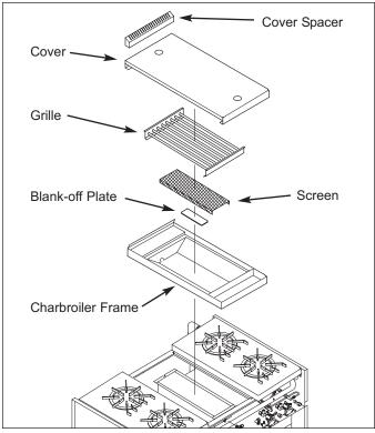
Figure 4-8. Components that Lift Off
