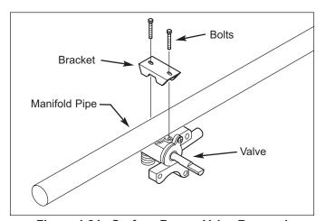
Figure 4-24. Surface Burner Valve Removal
