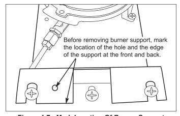
Figure 4-7. Mark Location Of Burner Support
