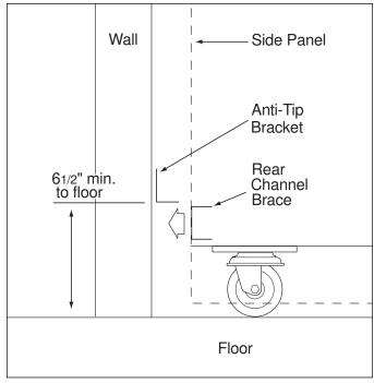
Figure 3-2. Anti-Tip Wall Bracket Installation
