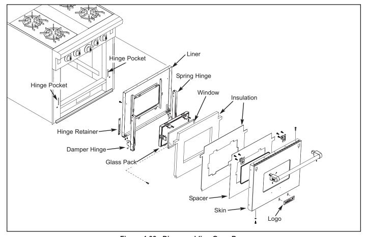
Figure 4-38. Disassembling Oven Door
