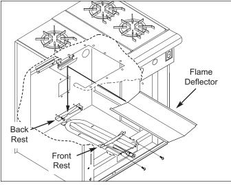
Figure 4-33. Flame Deflector Removal
