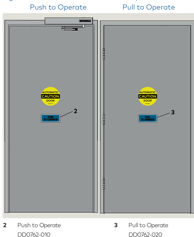
Fig. 5.2.1 Push / Pull initiation of door operation
