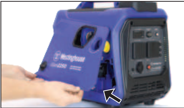
Figure 31 – Removing the LHS Maintenance Access Cover
