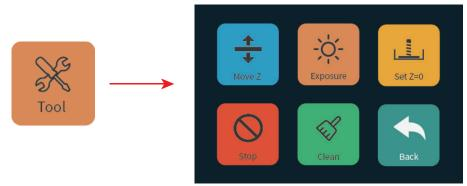
**Move Z:** Move the platform up and down along the Z axis
