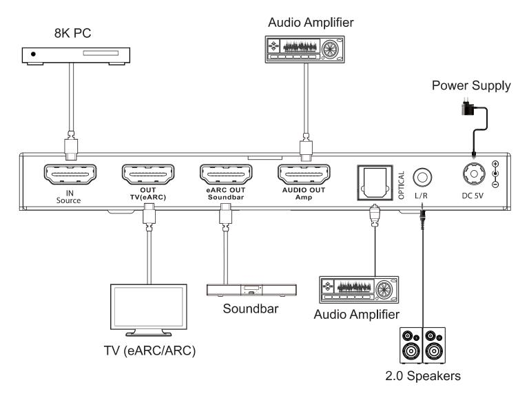
Note: When eARC/ARC mode is enabled, the audio signal of Amplifier/Soundbar is the audio returned from the TV. When eARC/ARC mode is disabled, the audio signal of Amplifier/Soundbar is from the HDMI input source.
