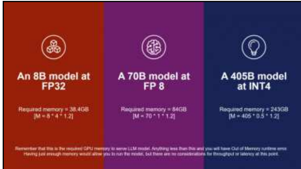
Figure 1: Example GPU Memory requirements for inferencing
