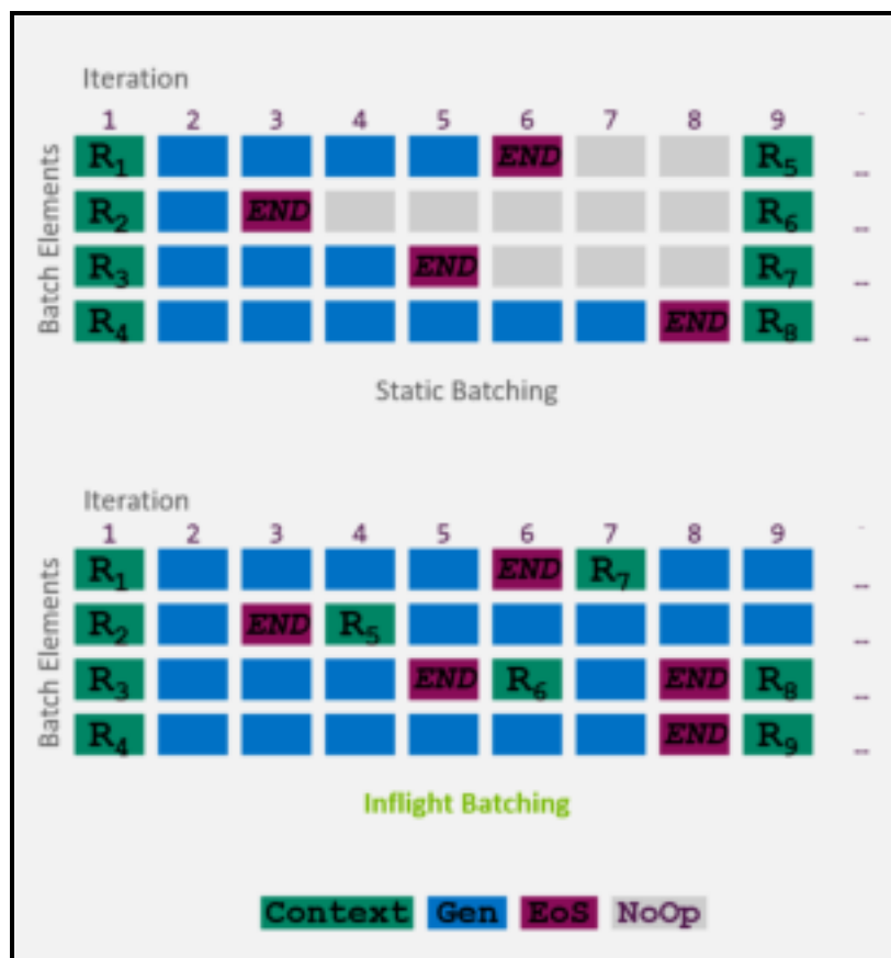
Figure 3: Inflight batching in action
