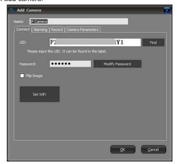
"Set WiFi": can setup camera to be connected via WiFi.
