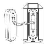
3. Pull out the fork connector cables and screw them to the back of the doorbell. Once connected, push the cables back in and click the doorbell onto the solar charger.
