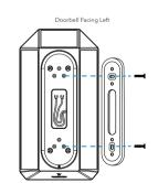
2. With 2 of the black screws provided, install the wedge plate (included with the doorbell) onto the solar charger. When the doorbell is faced on the right, install the wedge plate with the two screw holes on the left. When the doorbell is faced to the left, install the wedge plate with the two screw holes on the right.
