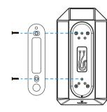
2. With 2 of the short black screws provided, install the backplate (included with the doorbell) onto the solar charger, inserting them into the middle screw holes.
