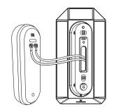
4. Pull out the fork connector cables and screw them to the back of the doorbell. Once connected, push the cables back in and click the doorbell onto the solar charger.
