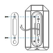
3. Insert 2 of the short black screws into the upper screw holes on both the top and bottom part of the backplate.
