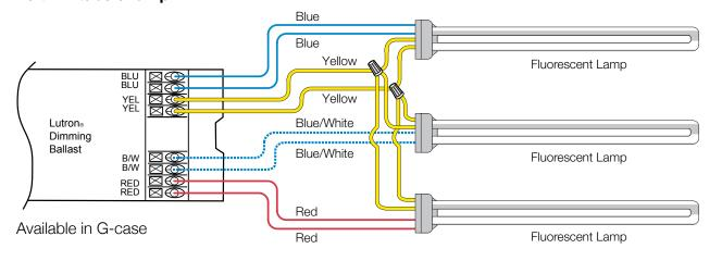
Note: Lamp terminals accept only one 18 AWG (0.75 mm²) wire. Ballast-to-lamp lead lengths must not exceed 3ft (1 m) for all wiring scenarios shown above.
