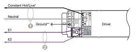
T-case can be grounded via case or ground terminal.
